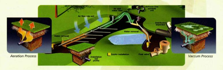
"The SubAir system allows us to pull water out of the greens when we get heavy rains and also allows us to blow air up through the green profile, to help cool down the soil in the greens during the summer"
